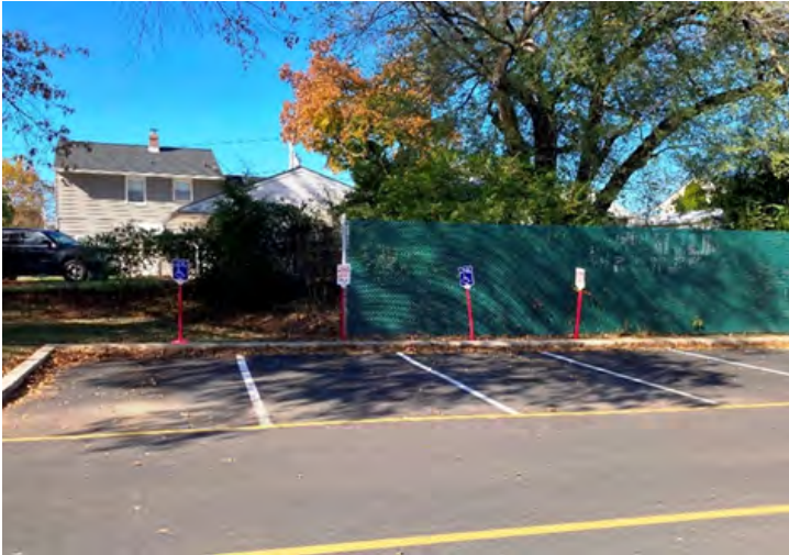
No access aisles, no nearby curb-cuts. (Polling Place: Baltz Elementary)
